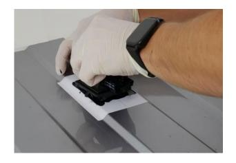
Glue on the roof duct Note the arrows on the roof duct and on the template
