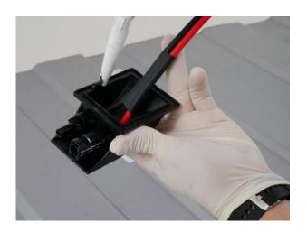
Apply adhesive as a closed adhesive bead Minimum adhesive layer thickness: 3 mm
